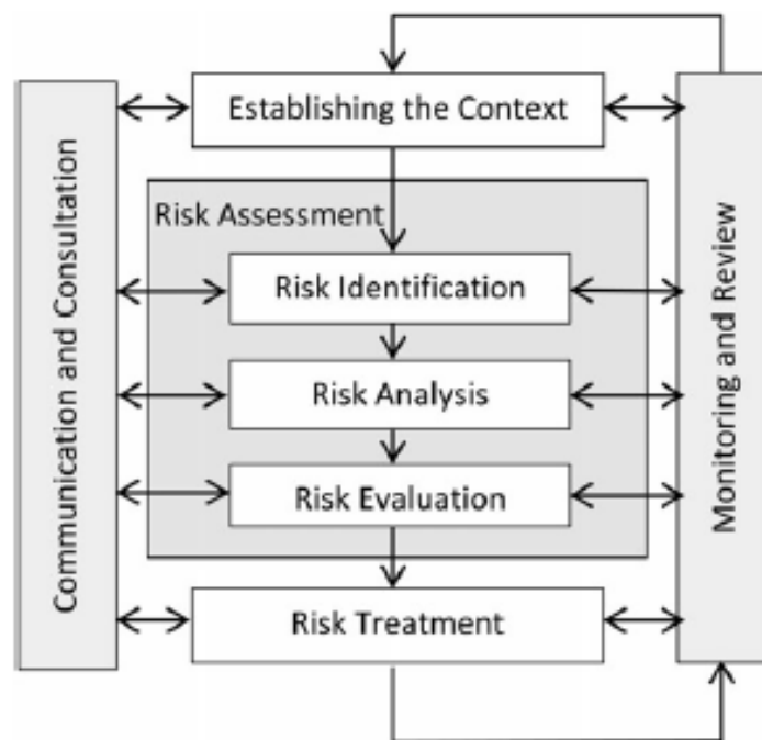
Figure 6.1 Position of risk assessment within the risk management process.
