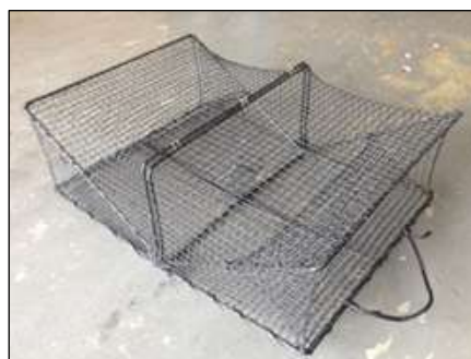
Figure 4.11. A box trap covered in one inch mesh trialled in near-shore marine waters and inland waterways of GB during June 2014.
