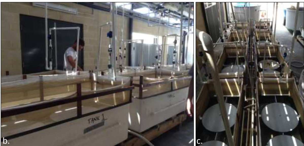
Fig 5.6. (a.) A schematic diagram of the coffin tanks used during the first and second aquarium trials. (b. and c.) The coffin tanks and circular PVC lids used to minimise disturbance during the first and second aquarium trials.
