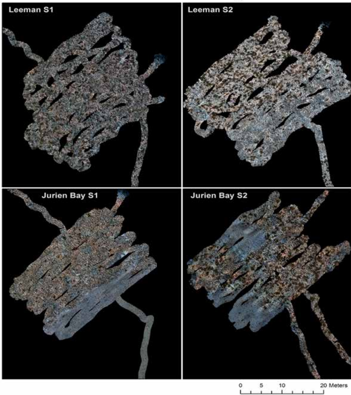
Figure 7.24. Examples of mosaics of 25m x 25m grids compiled from individual overlapping geo-referenced images collected by the AUV.
