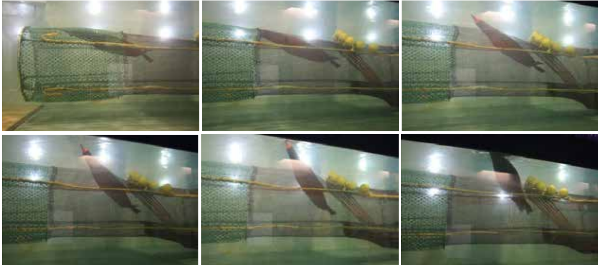
Figure 4. Sequence of photos taken during flume tank tests showing a performance evaluation of a megafauna replica passing through the top-opening escape slit (photos by J. Wakeford).
