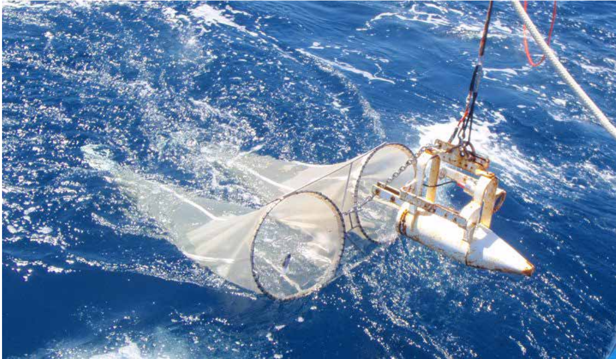
Figure 2.10 Towed underwater video downweight fitted with a 500 mm mesh plankton bongo net for benthic plankton sampling.
