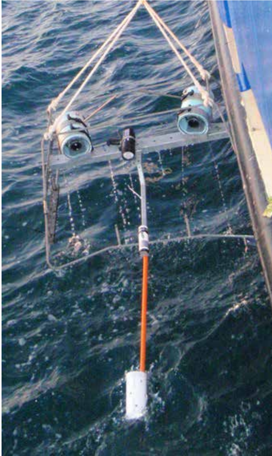
Figure 2.2 Stereo BRUV setup for night drop with light source (dive torch) attached to crossbar.
