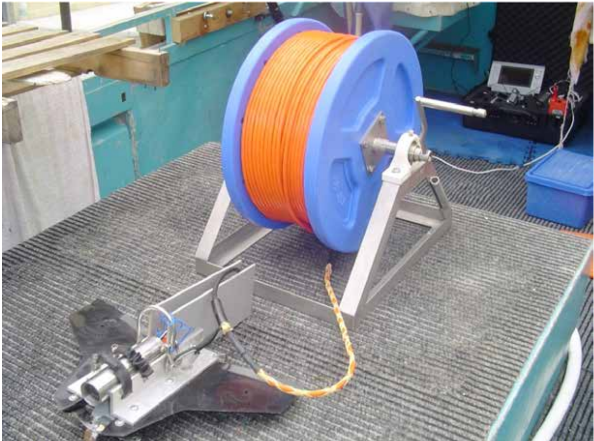
Figure 2.8 Towed underwater video systems for a) RV Naturaliste and b) RV Snipell .
