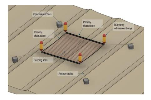
**Figure 1:** Proposed seaweed grow out panel consisting of seeding lines and anchor blocks.
