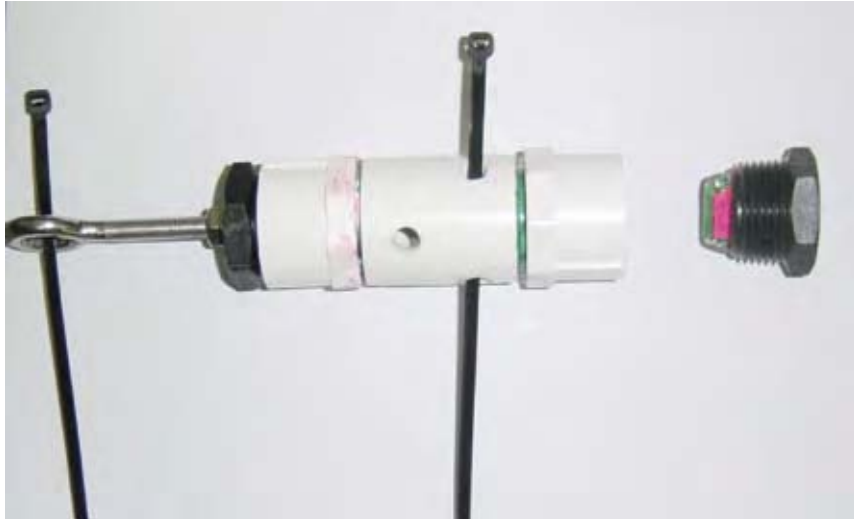
Figure 2 The casing used to protect and attach data logger to crab pot.
