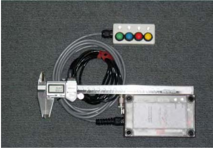
Figure 4.1 Electronic vernier calipers including data logger box with four data type options.
