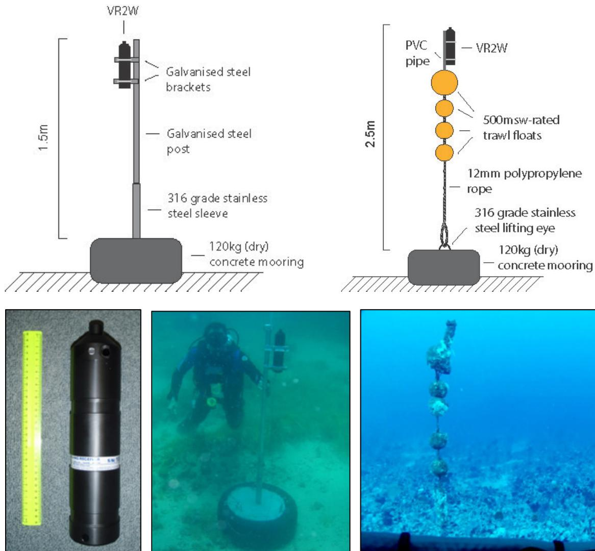
**Figure 5.** Diagrammatic views of diver-serviced (top-left panel) and ROV-serviced (top-right panel) VR2W installations; Vemco VR2W acoustic receiver (lower-left panel); diver-serviced VR2W mooring assembly (lower-centre panel) and deep-water (acoustic release) VR2W mooring assembly (lower-right panel).
