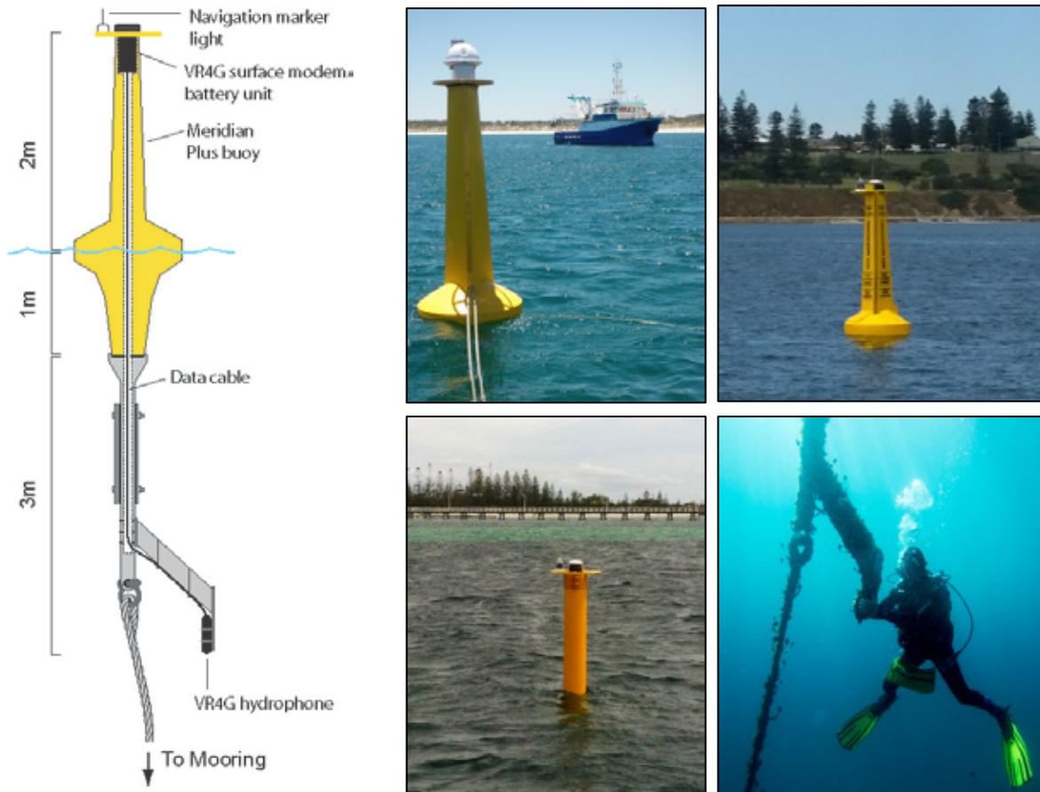
**Figure 6.** Cross-sectional diagrammatic view of a (third-generation) Meridian Plus VR4G receiver buoy (left panel, receiver components are coloured in black); prototype VR4G off Mullaloo Beach (upper-centre panel); Mk2 VR4G (in 3<sup>rd</sup> generation buoy) off North Cottesloe (upper-right panel); VR4G piling installation off Busselton (lower-centre panel) and diver inspecting hydrophone assembly on VR4G steel sub-frame (lower-right panel).
