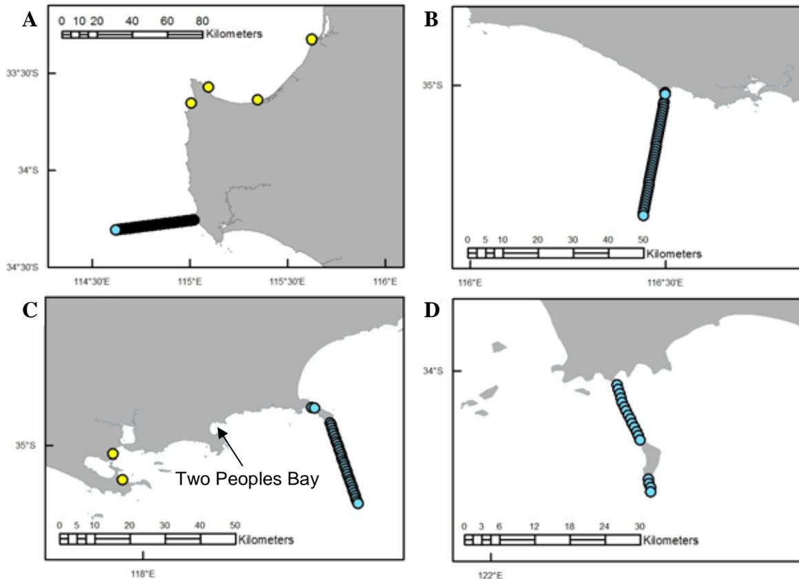
**Figure 7.** Locations and types of receivers deployed during the SMN operational phase (2012-2015) in (A) the Geographe Bay/Cape Naturaliste array, (B) Chatham Island array, (C) Albany and Bald Island arrays and (D) Recherche Archipelago array. Yellow circles indicate VR4G stations, blue circles indicate VR2W stations.
