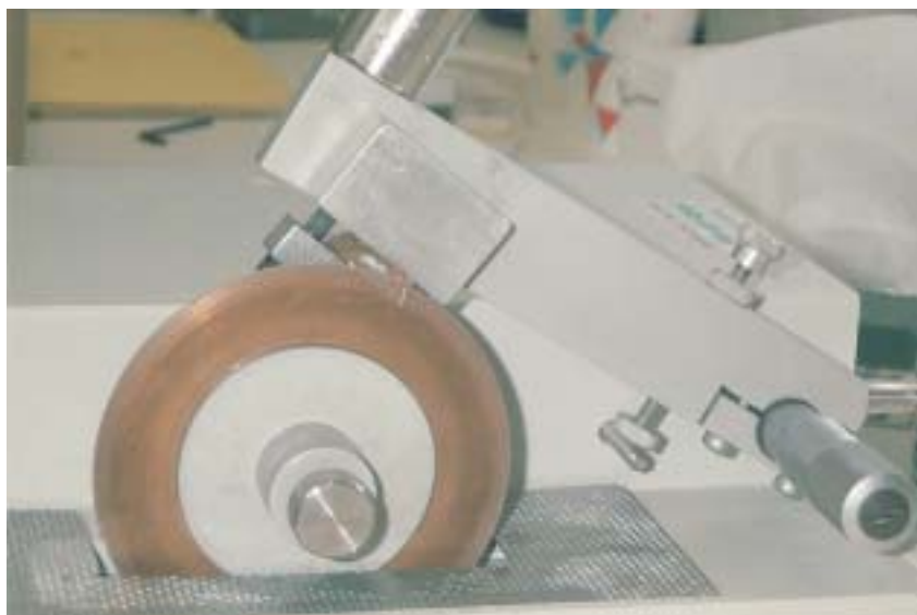
Figure 13. Cutting in process, showing chuck and otolith block angle in relation to the cutting blade.
