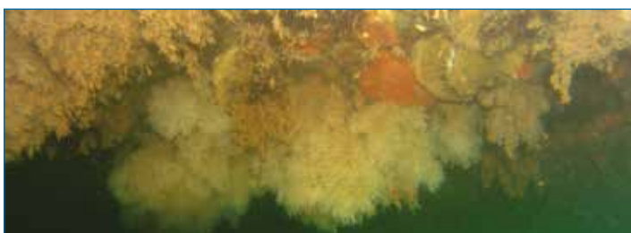
Hull fouling on the bottom of a dredge. Photo: Justin McDonald
