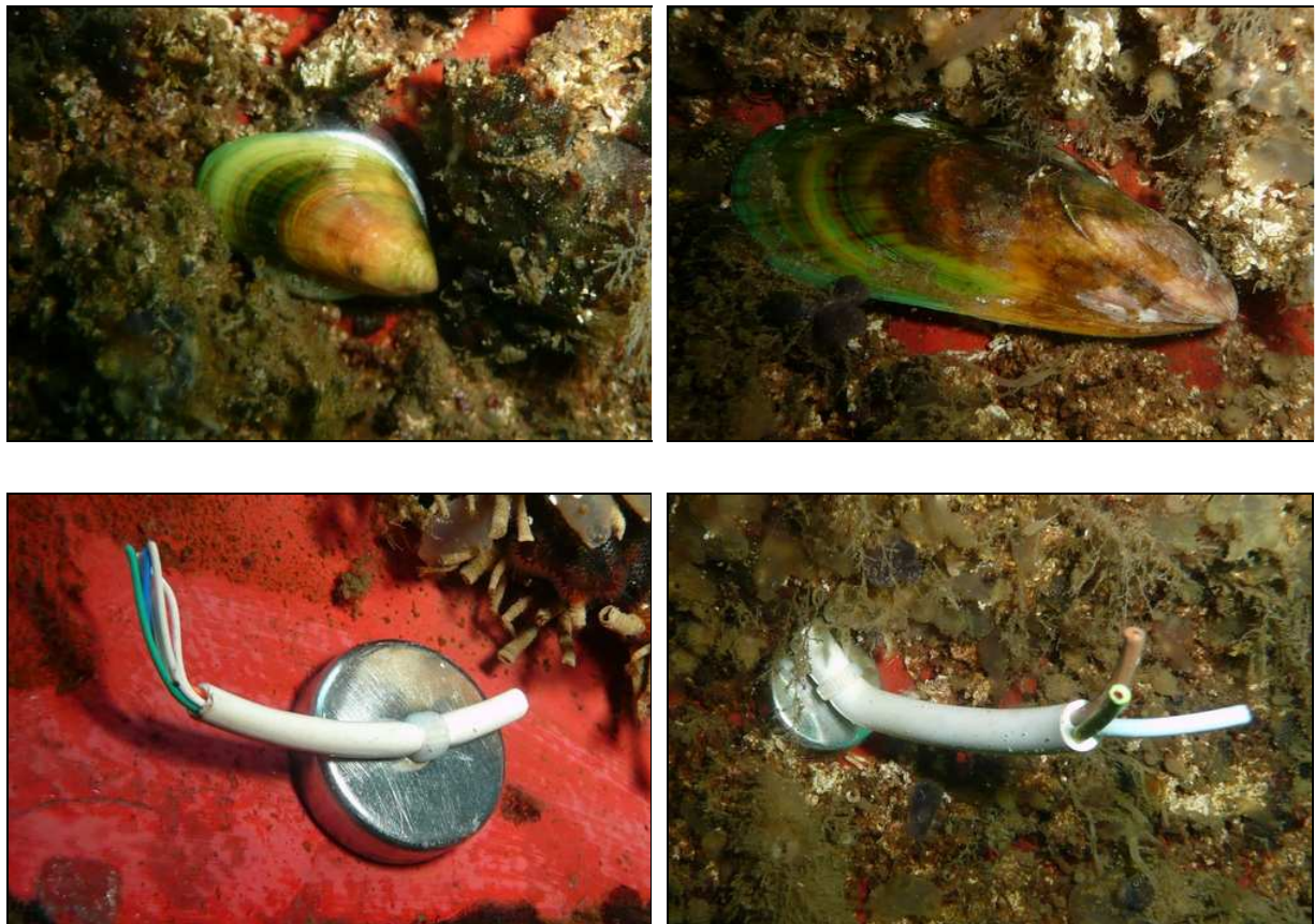
Figure 4: The various type and size of target IMS mimics used to evaluate the ability of the three methods to detect target IMS. Top = Asian Green Mussel look-alikes (left = small 15-20 mm; right = large 60-90 mm); bottom = invasive tubeworm look-alikes, (left = small 20-30 mm; right = large 60-90 mm).
